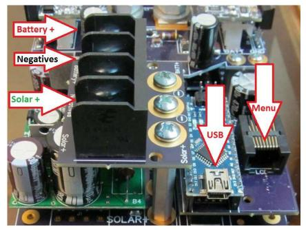
The MP-20 uses a four position terminal block located inside the unit for the power wire hookup. The top position is for the battery positive. This wire should be run directly to your battery positive post (or positive buss bar) via a breaker or fuse. <u>A breaker or fuse is required for all wires</u> leaving an energy source.
